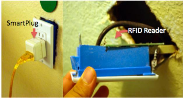
figure 1. The implemented SmartPlug in the GTSH.
