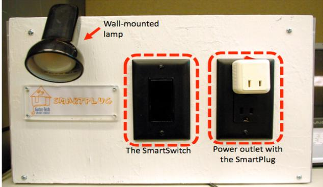
figure 2. Front side of the SmartPlug and SmartSwitch for demonstration.
