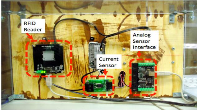
figure 3. Back side of the SmartPlug and SmartSwitch for demonstration.
